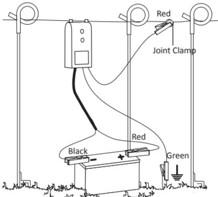
The Energizer can sit on a fence line using the hooks at the top of the enclosure.
